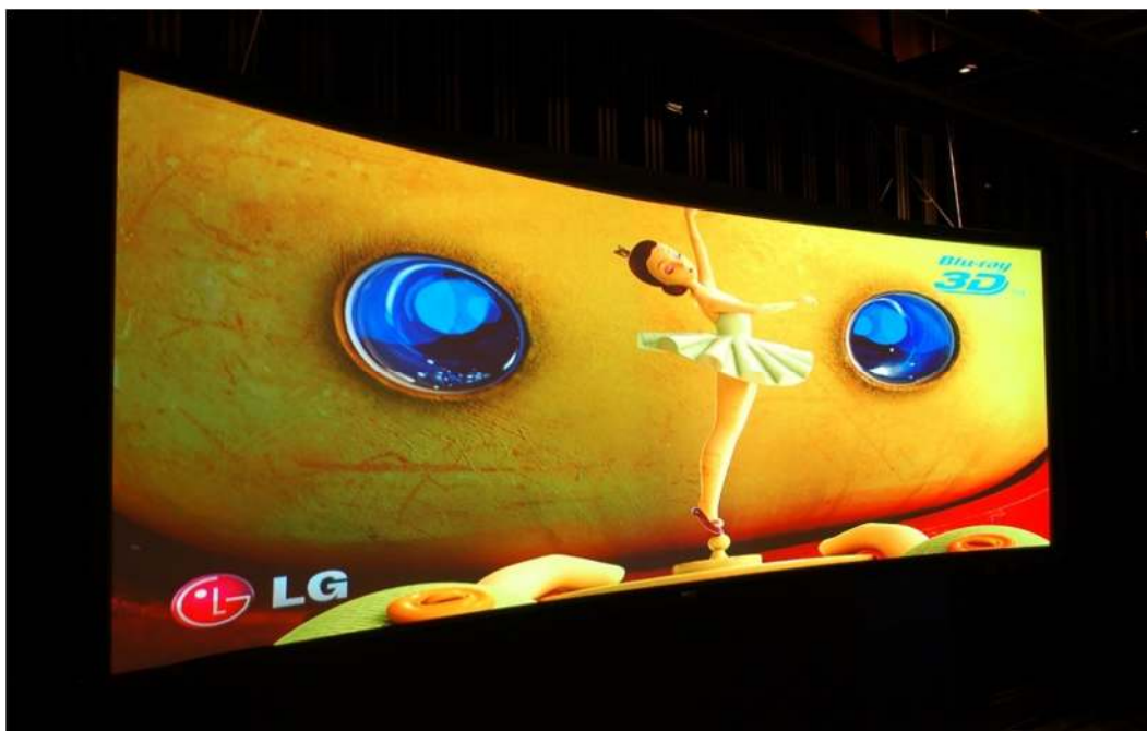
(4x Epson full HD projectors to do edge blending on curved screen for passive 3D display)
